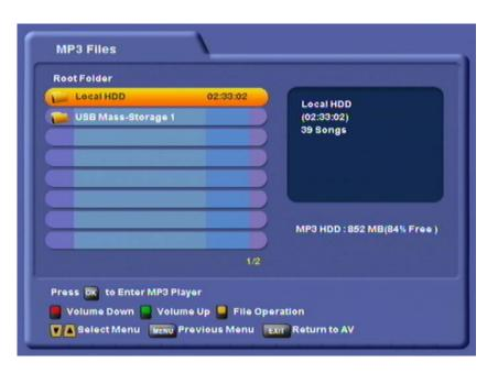
Use the A v buttons to select the desired directory and press v to open the directory and access its subfolders. In the above example the first directory listed is the local hard disk of the UFS 821 (Local HDD). The second directory is a USB memory stick. You can also access an external hard disk via the USB port on the UFS 821 and open files on it without having to save them to the UFS 821.
